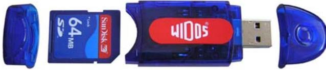
Remove the rear cap and plug card according to the image into the USB card reader.
