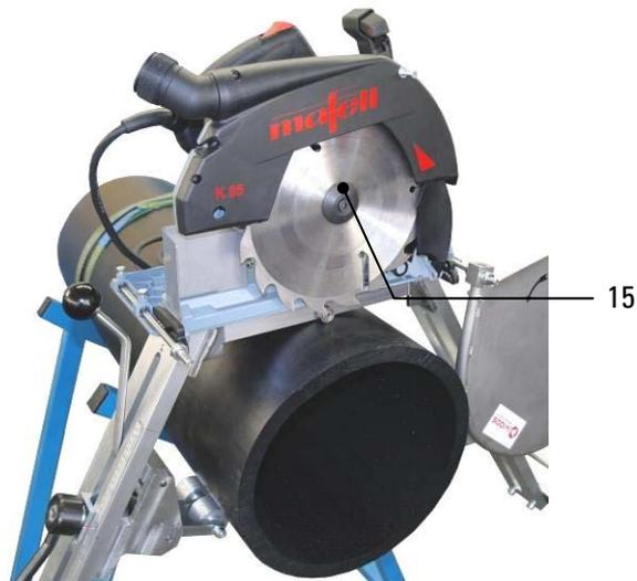
Take the attached Allen key SW 5 and detach screw (15) of the saw blade.
